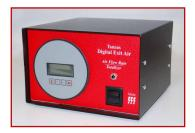
The use of an exit air device is required in D892 to measure the total air volume that has passed through each gas diffuser during the 5-minute blowing period — unless the operator choses to run according to the Alternative Procedure per Section 11 of the D892 method. The Tannas Digital Exit Air Device is the best alternative for this measurement. Tannas also offers a more basic Inverted Cylinder device at a lower price point. Contact us for details.
